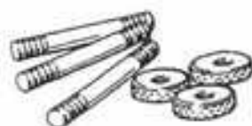
Fig.3 The C.300 Stud Clamps and Nuts. The stud clamps are in four heights to suit up to 2½" moulds. The longest stud (C.252 'D' Stud) is ¾" long and is threaded down one end for over 7/8"; you can cut and tailor it to the length you want.
