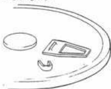
Fig. 15 The component shown in Fig. 14 has been cut in two for casting; it can subsequently be glued or soldered.
