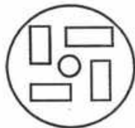
Fig.10 Items laid up in the modelling material at a tangent to the centre - this layout will be correct in the mould.
