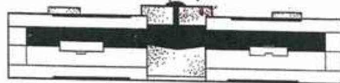
Fig.20 The first half of the mould - the bottom half (shown black) finished (see also Fig.7a)
