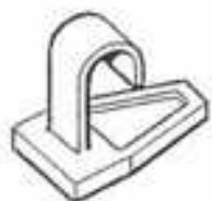
Fig. 14 Showing undercut where rubber could be locked in.
