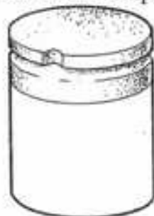
Fig.33 Fence removed, channel cut round, and notch cut.
