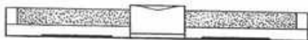
Fig. 12 Ring is filled level with Chavant modelling material ready for embedding the pattern. Note that plug 'A' is proud in the middle.
