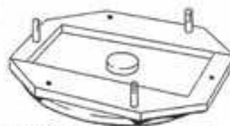
Fig.4 Economould Frame set up ready to use (first half). Each frame is in two identical parts - 4 parts to a set.
